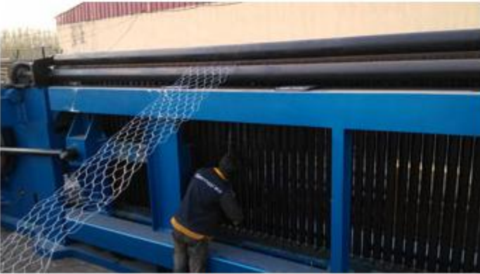
Gabion mesh machine adjusting
