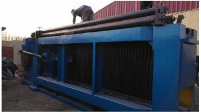
Gabion weaving machine
